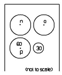
These are driven by a wheel on a third shaft p which in turn is driven by a 30 wheel on a shaft carrying a handle.
